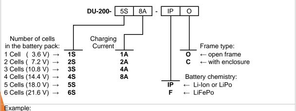
A DC-UPS module for 5 cells Li-lon battery pack with a charge current of 8 Amperes and without enclosure has the following part number:
